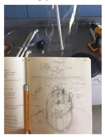
Fig 3. This is the original design for how the tank would function. I incorporated all of the information gained from researching my target species to ensure the aquarium would make a safe habitat for soft bodied larvae.
